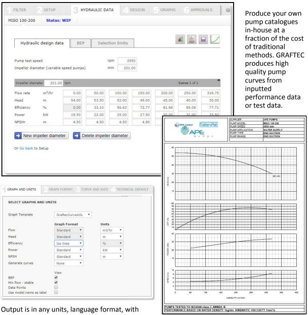
Output is in any units, language format, with automatic plotting of Iso-efficiency and Iso-power lines.
